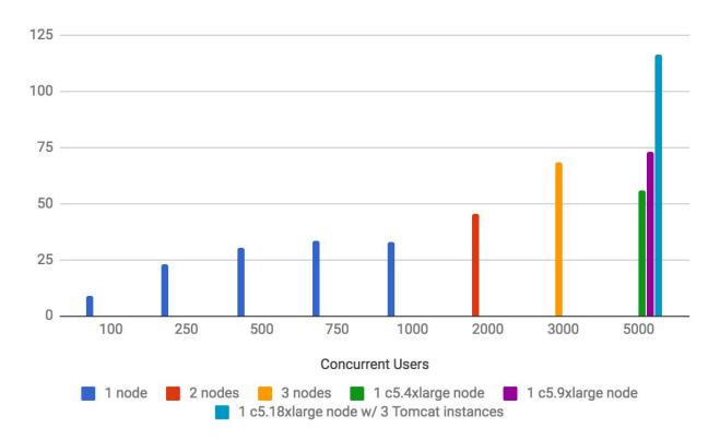
In terms of throughput, a single c5.large node (2 vCPU, 4GB RAM) maxed out at about 33 requests per second at 750 concurrent users. When the concurrent users increased to 1000, the throughput remains about the same.
