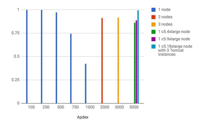
For a single c5.large node (2 vCPU, 4GB RAM), the Apdex dropped once it reached 1000 concurrent users. As before, scaling out by adding nodes did maintain an acceptable an Apdex value. The single c5.18xlarge (72 vCPU, 144GB RAM) node with 3 Tomcat instances was able to achieve a 0.995 Apdex value with 5000 concurrent users.
